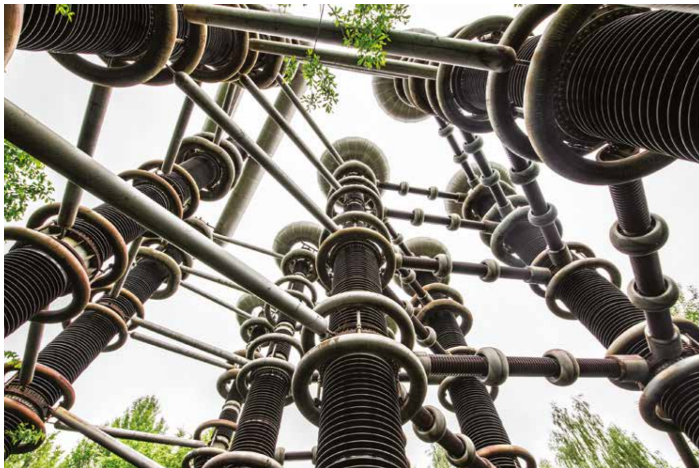
Prototype of a Tesla coil installed at the end of the 1970s in a research centre that was secret at the time. It was used to test insulators for the protection of vehicles, aeroplanes and electronic equipment against lightning.
